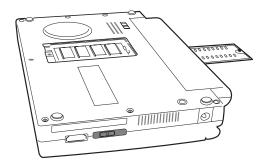
Sample removing the memory module slot cover
